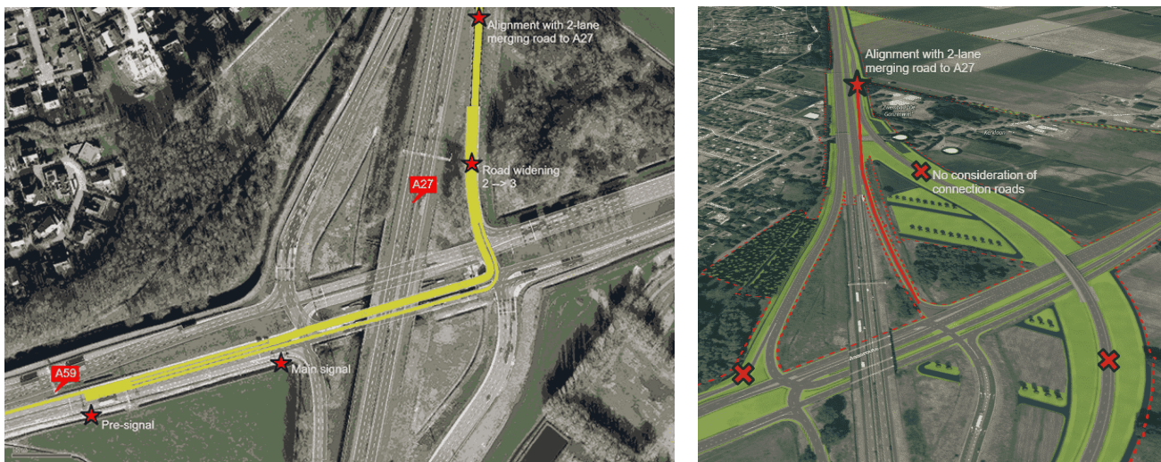
Figure 5.5. – Road Section That Facilitates a Pre-Signal System Size of 3 Lanes in Left-Turning Direction (left) and Alignment With Construction Design (right)
