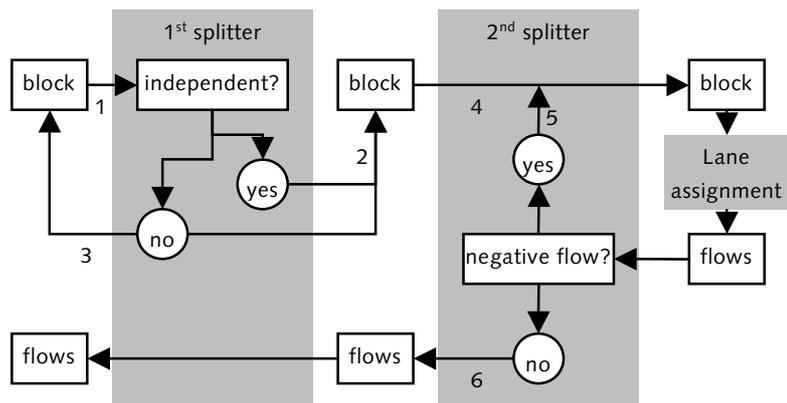
The first splitter splits blocks independent of flow, and it is therefore not needed to apply the first splitter every time step. Instead, split locations will be stored during the model initialisation.
