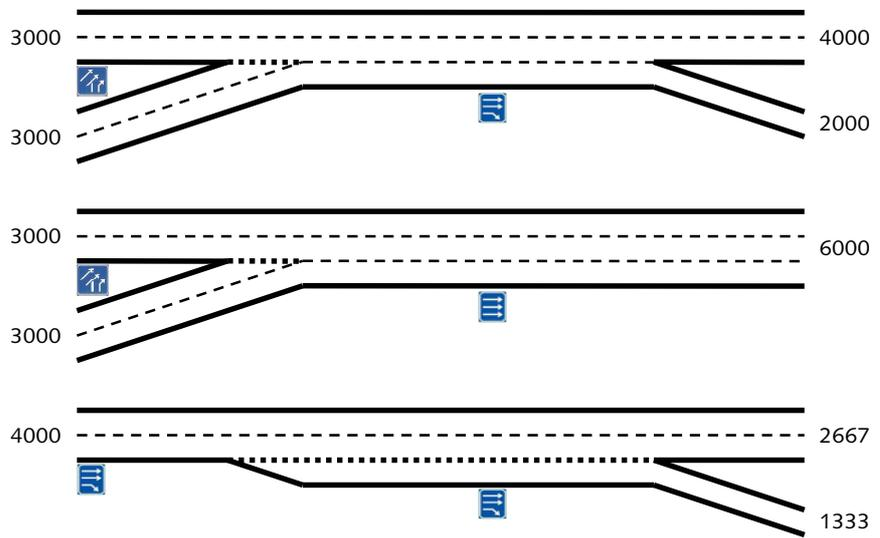
1. The shockwaves and congestion and spillback observations from controlled intersections also hold for weaving sections. The link with spillback is however either the off-ramp or the highway itself for the merge section. Despite the under saturated condition of the links, all layouts have congestion at the weaving section before there is spillback. Even the off-ramp, which is an additional lane, creates congestion. The amount of congestion is however less.
