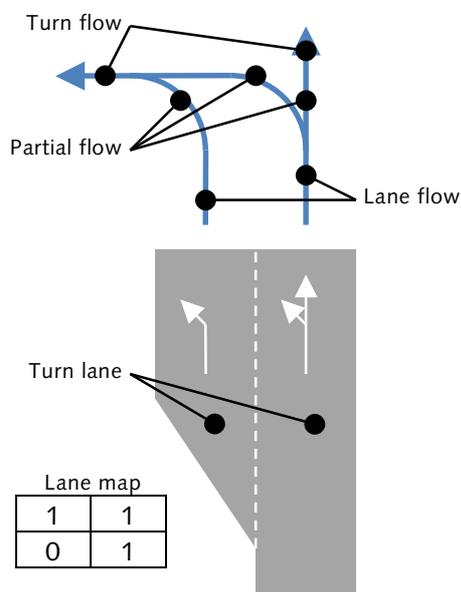
A *turn flow* is all flow from one link to another. A *turn lane* is a lane at the end of a link that can be used to turn certain ways over the node. *Lane flow* is all flow from a turn lane. *Partial flow* is part of a lane flow belonging to a specific turn flow.
