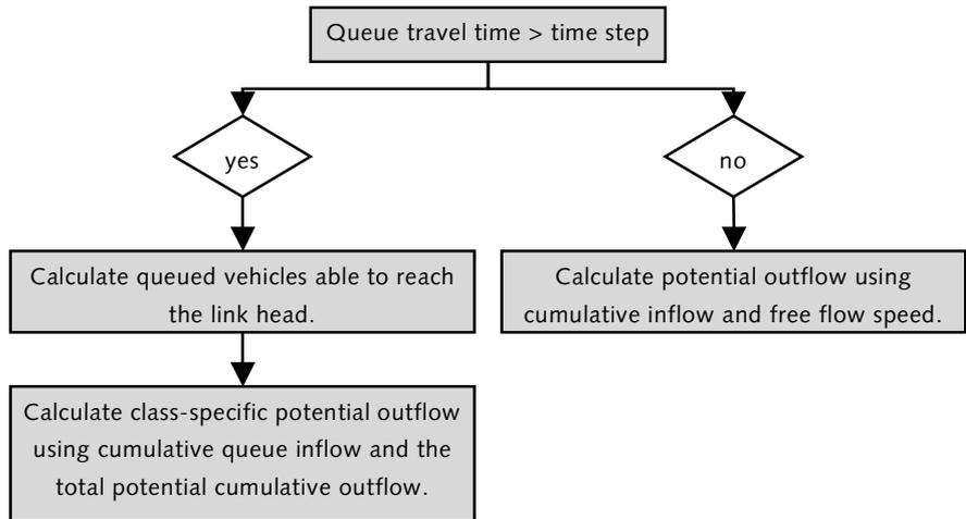
Figure 5.5: Option 2 to calculate  $V_a^{q'}$ .
