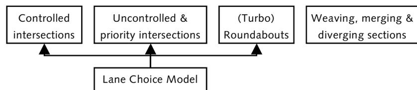
The current node model in EVAQ will stay active, as maximum link inflow still needs to be balanced with potential link outflow. The new node models will limit flow further if constraints are violated. The order of practice will be:
