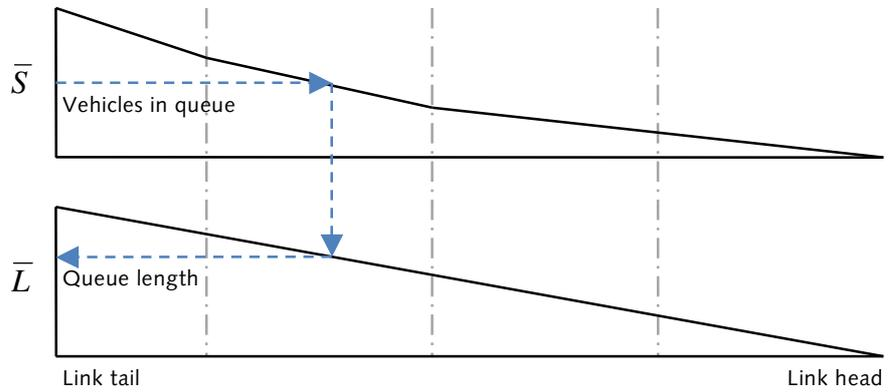
With the queue length, cumulative queue inflow until the next time step ( $Q(t+1)$ ) can be calculated in the same way as in the original model using linear interpolation over link inflow, see Equation A.13. All information to calculate maximum inflow and potential outflow is now gathered. Queue inflow is known, completing the set of flows that make up the link model.
