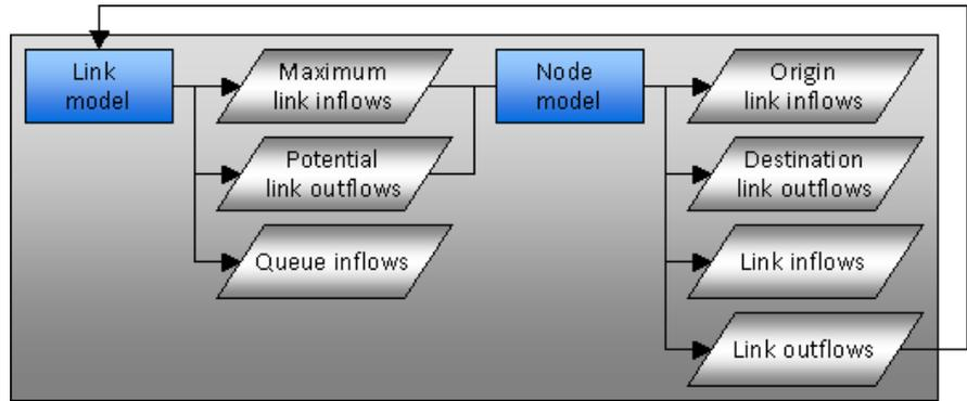
The complexity of the framework has reduced, but the individual modules will increase in complexity. The link model defines the queue as multiple cell states based on past outflows instead of a single constant state. The node model will additionally check constraints on the node.
