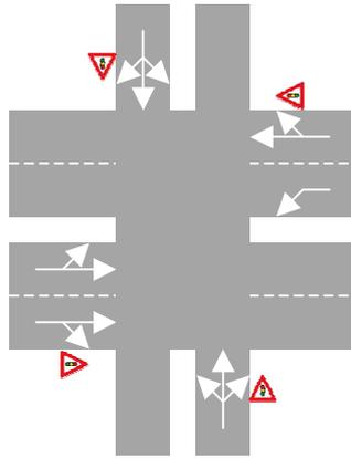
lanes. Capacity equals 2000 pcu/h/lane and saturation flow equals 1800 pcu/h/lane. From the north and the south 1000 pcu will leave evenly spread throughout an hour. For the east and west this is 2000 pcu.
