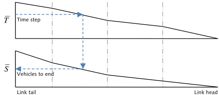
Different from existing models is the fact that the cell states are aggregated into cumulative quantities per link, providing an easy and fast way to derive momentary maximum link inflow and potential link outflow. Dynamics for each cell pair do not need to be assessed.
