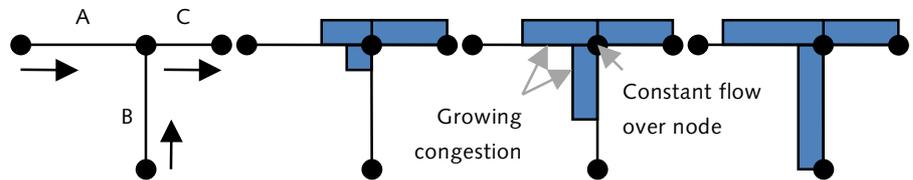
The steps between the horizontal parts can be explained in relation to the spillover. As soon as a link is spilling back, flows of upstream links will be reduced. The opposite happens if spillover disappears. Flows of upstream links will then increase if demand is still present.
