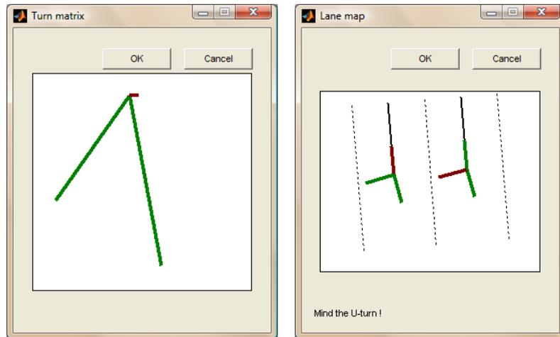
By clicking on a turn direction in the pop-up window, the turn will be enabled (green) or disabled (red). In Figure B.2 (left) the U-turn from and to the north is disabled. Click 'OK' in the pop-up window to accept any changes. This process needs to be repeated for every link from which turns are impossible. If all turns are possible, select the 'All' option.
