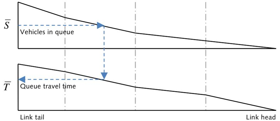
The time remaining ( $\Delta t'_a$ ) for the free flow section is given by the time step minus queue travel time.
